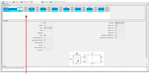
Select the appropriate tools for the different forging operations that you have to perform in order to get the given forge piece. Your standard tools will be pre-selected.
